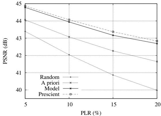
Fig. 4. PSNR as a function of the PLR for the *elephantsdream* video sequence, 70% sent as loss-free service.
