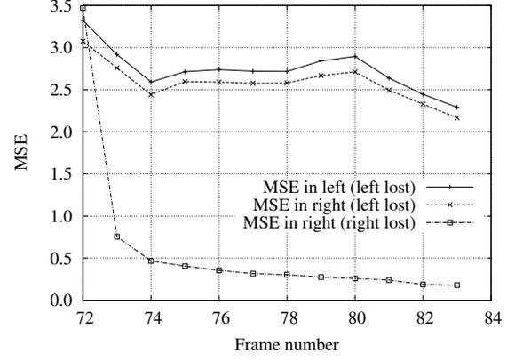
Fig. 2. Distortion (MSE) introduced in the left and right view of a GOP if the first left or right frame of the GOP is lost. Interview sequence.
