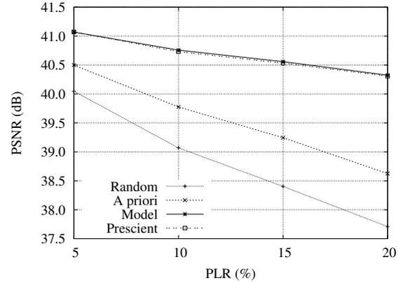
Fig. 5. PSNR as a function of the PLR for the *ballet* video sequence, 70% sent as loss-free service.
