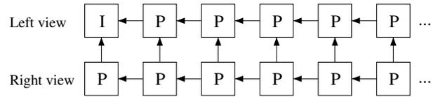
Fig. 1. Encoding dependencies for a stereoscopic low delay scenario.
